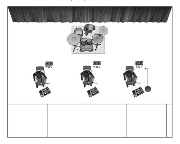
All the electric equipment must be grounded and powered no less than 220 V. It's necessary power (230 V) sockets for each cello player for the adaptors for their sound processors- two (2) cockets for each, and at the drummer position- two (2) minimum. Please provide three (3) chairs without arms for cello players . We will change technical specifications according your venue, stage size, show specific and technical possibilities, but ONLY with management and sound engineer agreement.
